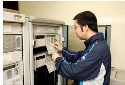
Observatory staff inspecting the operation of the caesium beam atomic clock
