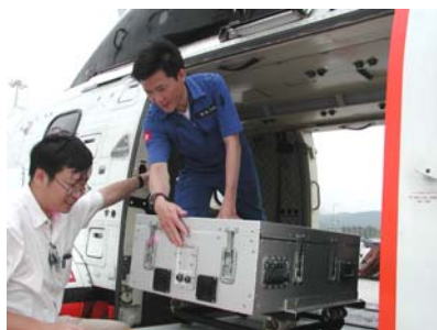
Observatory staff installing the aerial radiation monitoring system onboard a Government Flying Service's helicopter
