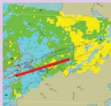
Figure 2 Display showing windshear ("bandaid"-shaped areas in red) and rain echoes detected by the Terminal Doppler Weather Radar at 9:55 a.m. on 24 June 2005.
