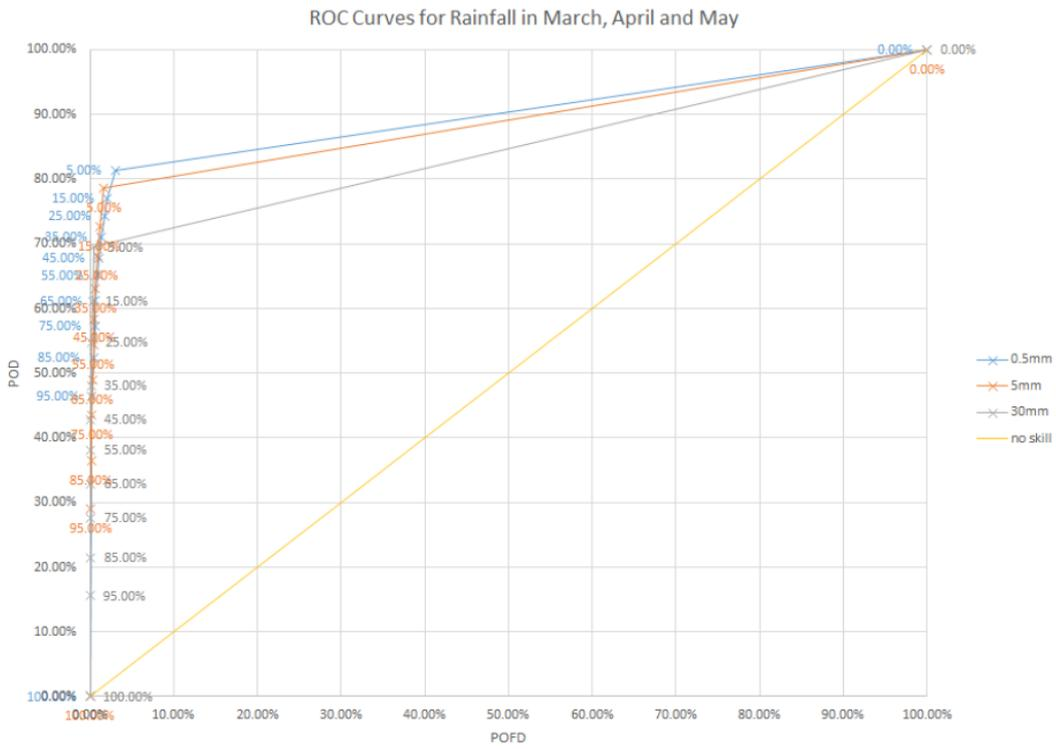
**Figure 7.** The ROC curve of the probabilistic rainfall nowcast in the spring of 2014.
