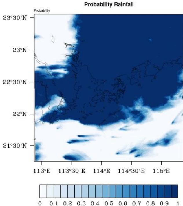
**Figure 4.** A forecast hourly probability rainfall nowcast contour map with 0.5 mm/hour as rainfall intensity threshold, based at 23:00 on 8 May 2014 (HKT).
