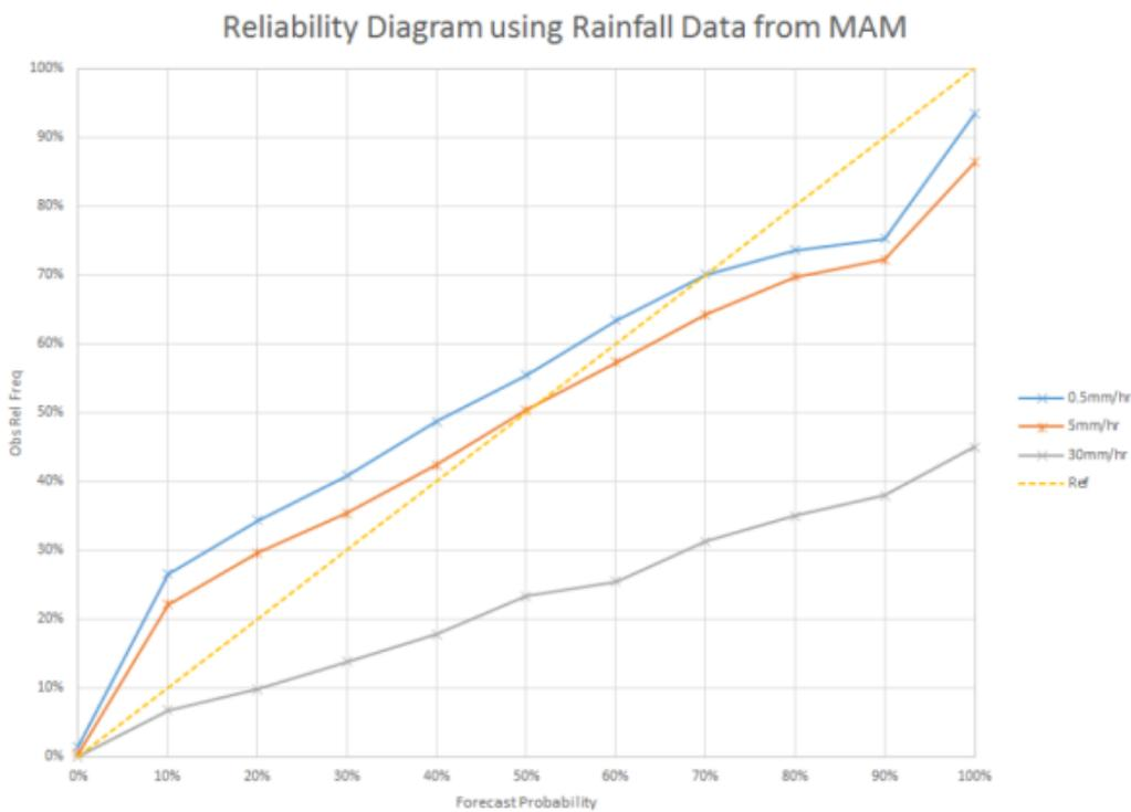
**Figure 6.** A reliability diagram constructed with probabilistic rainfall nowcast in the spring of 2014.
