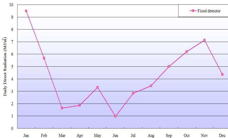
Figure 4 Average daily direct solar radiation levels to be received by a surface mounted at an optimal orientation of 120^\circ and tilting angle of 40^\circ , based on measurements at King's Park Meteorological Station, 2009.
