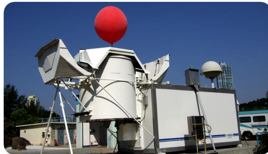
京士柏氣象站自動高空探測系統 Automatic Upper-air Sounding System at King's Park Meteorological Station
