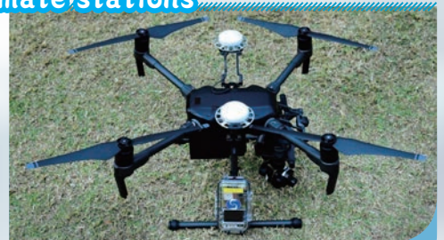
Microclimate sensors on a drone
