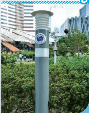
Microclimate sensors on a bollard
