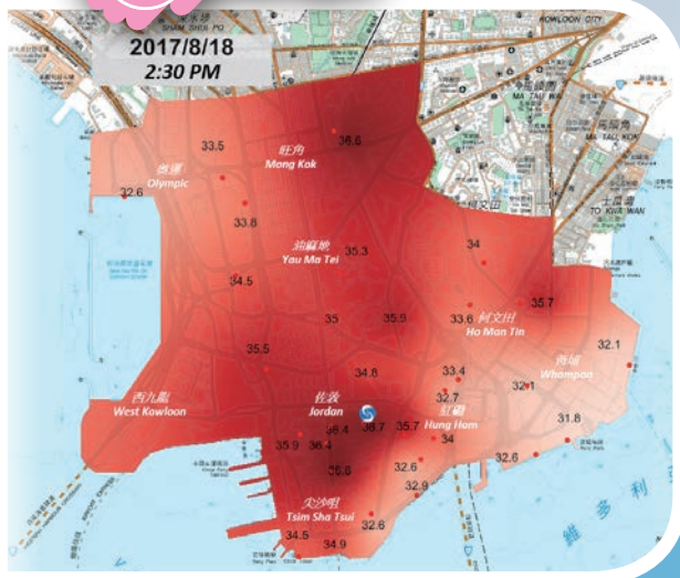
Results of a microclimate study conducted in Kowloon Peninsula: under the influence of easterly winds, the temperatures over the eastern part of Kowloon Peninsula are generally lower, while the temperatures over the central and western parts are somewhat higher.
