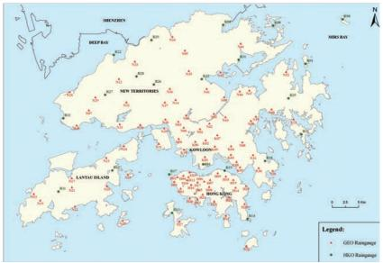
*Figure 5: Locations of GEO raingauges and HKO raingauges in Hong Kong*
