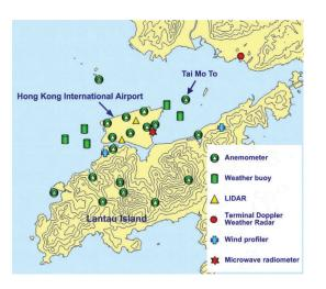
Based on real time data from detection systems, the broad prevailing meteorological conditions, aircraft reports and data, the HKO issues windshear and turbulence alerts and warnings. Alerts are relayed by air traffic control personnel to aircraft landing at and departing from the airport. Warnings are provided to aircraft on Voice- and Digital-Automatic Terminal Information Service (ATIS).
