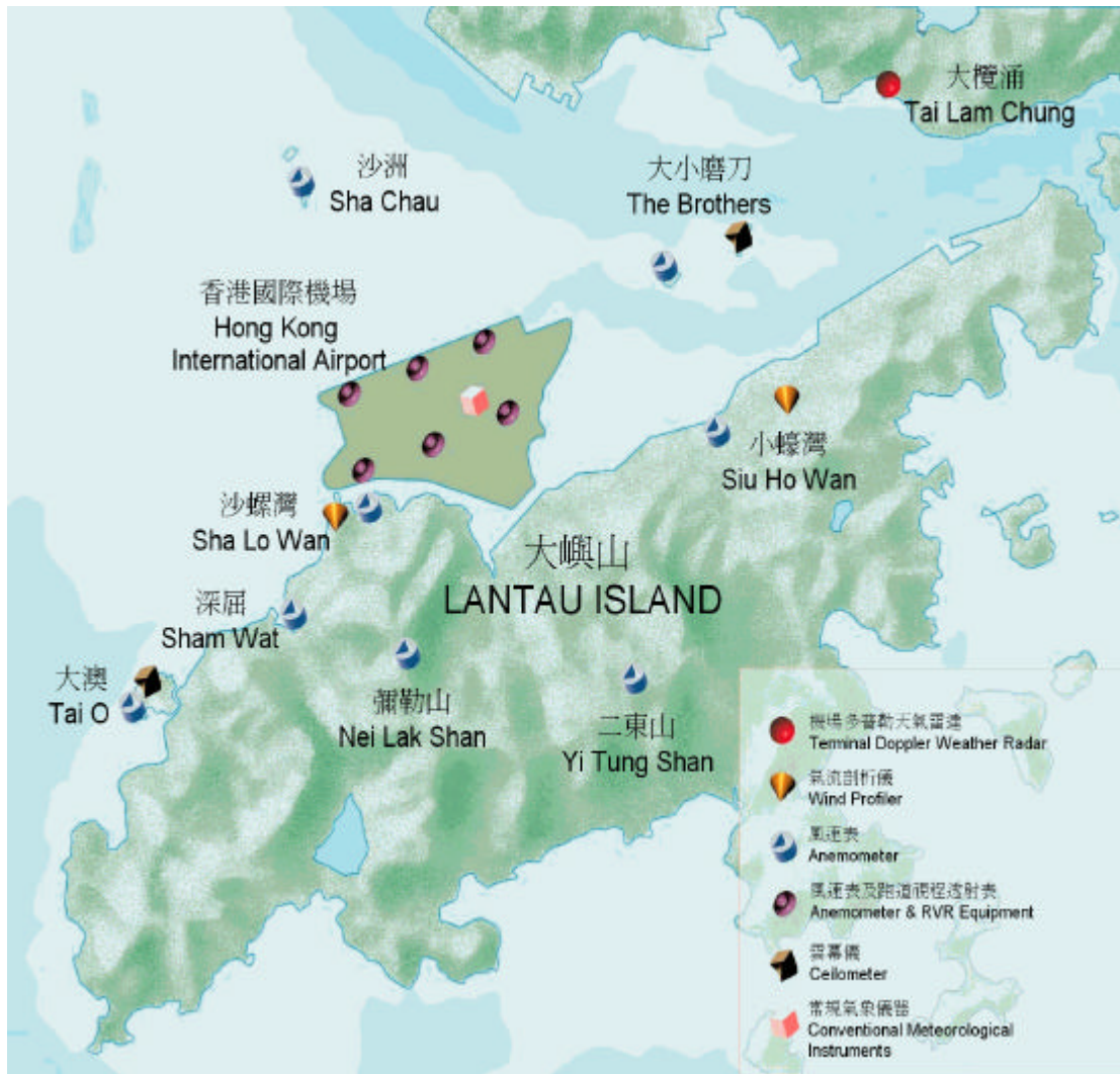
Figure 4 Network of weather sensors for the Hong Kong International Airport.
