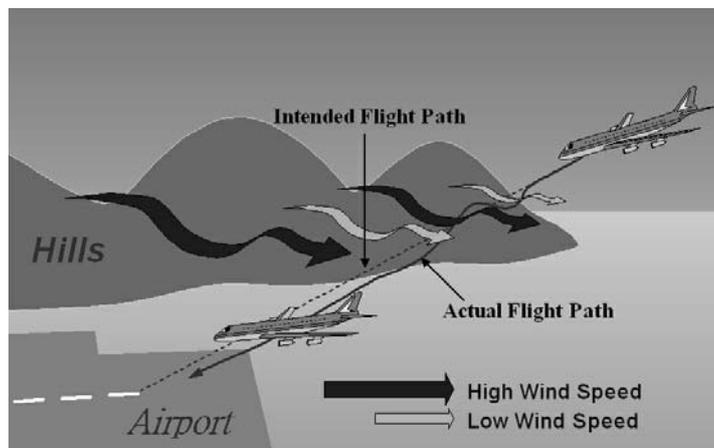
Figure 3 — The most common cause of wind shear at KHIA is the terrain-induced airflow pattern.
