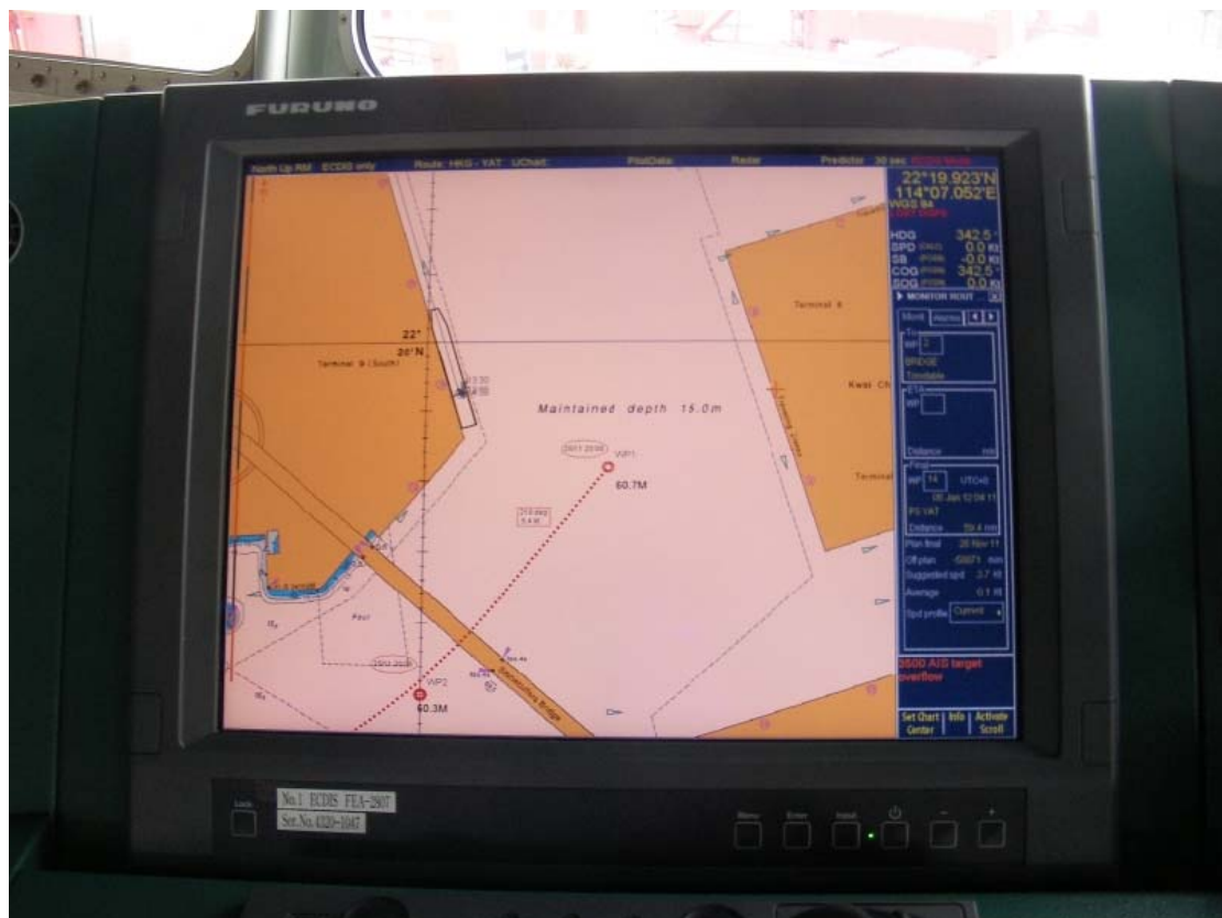
Figure 2 Monitoring of the water depth from a sea-going vessel
