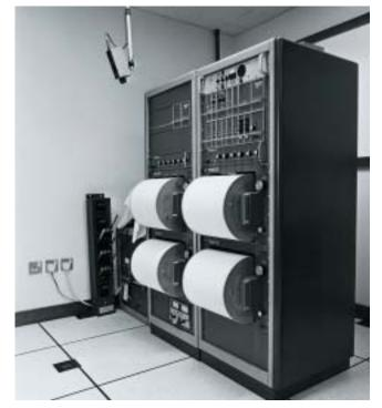
Fig. 3.44 Seismographs housed inside the Observatory's seismological laboratory. Courtesy Hong Kong SAR Information Services Department
